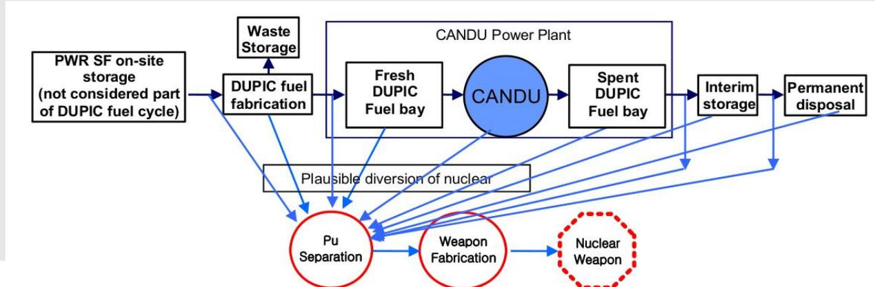
DUPIC material flow, possible diversion points, and coarse pathways considered [Fig 5., IAEA-TECDOC-1684]
